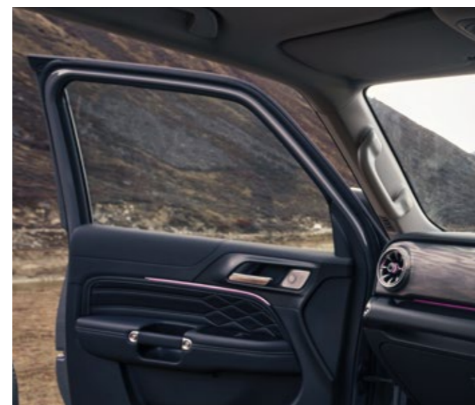
DOUBLE-LAYER ACOUSTIC GLASS TO ENHANCE NVH LEVELS
